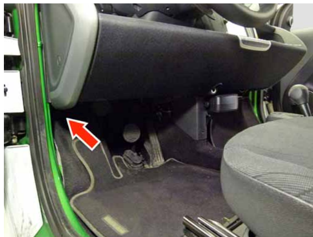
High-voltage disconnect located in driver-side footwell
